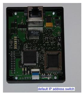
In order to set default IP address, to turn switch to right position and then you must apply the power supply.
