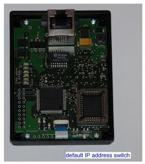
In order to set default IP address, to turn switch to right position and then you must apply the power supply.
