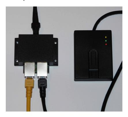
EFIS121 Fingerprint Scanner is powered over the Ethernet cable (Figure 1). Black box with 2 Ethernet inputs provides DC power to the scanner (black cable on the picture) and at the same time connects EFIS121 to the network (yellow cable on the picture). It's possible to use 2 types of passive PoE adapter.
