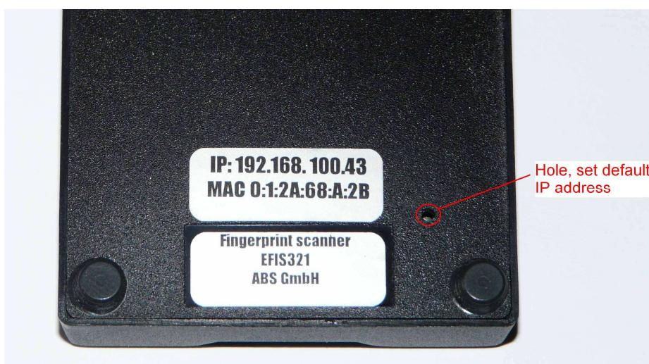
In order to set default IP address, press the button via hole and keep of it for 2-3 seconds. The EFIS321 scanner must be connected to power line in this time.
